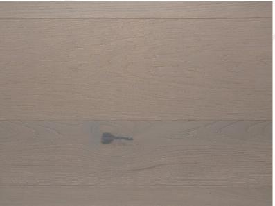
Oak plank in 3-layer construction with small bevel on long side and approx. 4 mm top layer, with approx. 4 mm backing in the same wood and middle layer conifer. Tongue and groove on all sides for easy installation. Cracks, knotholes and large knots are emphasized with black putty. Variations in colour and sapwood at the edges possible. Small open cracks and unsealed spots of a few millimetres are permitted.
