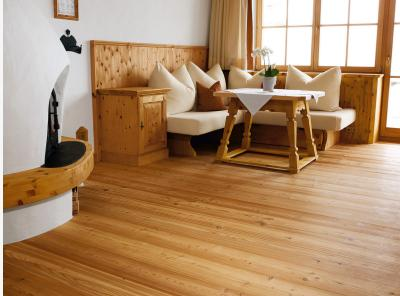
Close-grained larch plank in 3-layer construction with small bevel on long side and approx. 4 mm top layer, with approx. 4 mm backing in the same wood and middle layer conifer. Tongue and groove on all sides for easy installation. Knots up to 50 mm diameter and splay knots (30 x 60 mm) are possible. Max. 4 pitch pockets per plank are permitted, also cracks up to 50 cm. Some sapwood is possible. Small open cracks and unsealed spots of a few millimetres are permitted.
